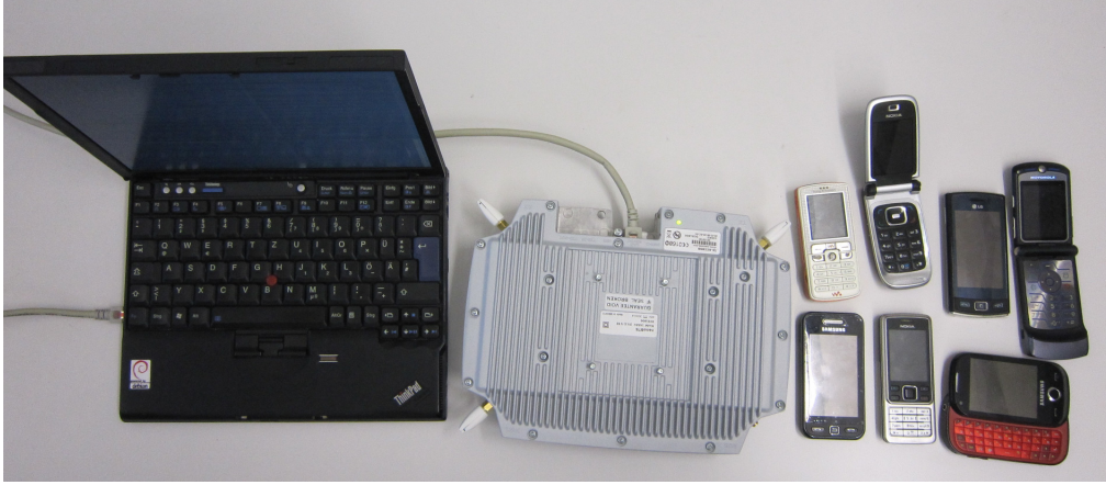
Figure 1. Our setup: The laptop that runs OpenBSC and the fuzzing tools, the nanoBTS, and some of the phones we analyzed.
